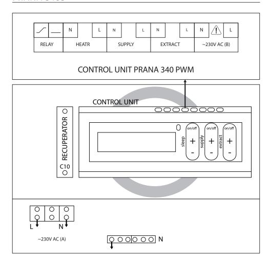
Terminal (~230V AC (A)): power supply connection ~230V.
