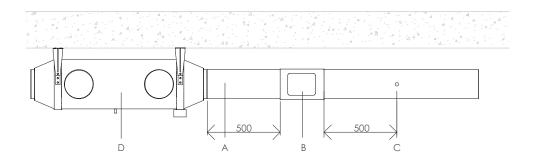
Schematic diagram of installation of a duct temperature sensor.
